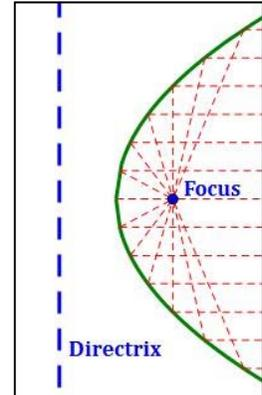
In the diagram, the red lines approach the parabola from the right, reflect off its surface and meet at the focus. This is how satellite dishes and parabolic antennas work. A paraboloid (a 3D version of the parabola) provides a wide area from which to collect signals. The signals reflect off the paraboloid surface and meet at a receiver placed at its focus, thus significantly amplifying the signal.
